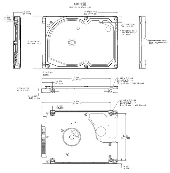
Figure 5. Mounting dimensions—top, side and end view
